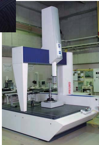
三次元测定器进行形状测定 Profile measurement using a coordinate measurement machine
