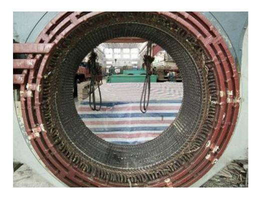
Exciter's stator coil damage due to chamber scratching; All rotor's fan blades broken;
