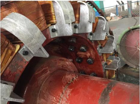
All dumping rings broken; 2 transformers in terminal box spark through;
