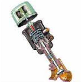
The disc's parabolic shape of the 2-way control valve series 290 PD ensures a Kv proportional to the opening of the valve
