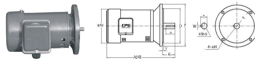
適用機型 APPLICABLE MODELS : CV..AT, CV..ATB, CV..A, CV..AB
