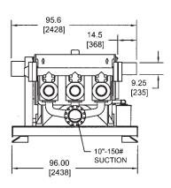
Note: All installations must contain a pressure relief valve in the discharge line near the pump.
