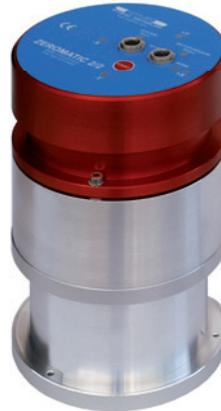
The two-dimensional inclination measurement sensors ZERO-MATIC 2/1 and 2/2 are perfectly suited for any application where monitoring of the smallest changes in absolute inclinations over a longer period of time is required. The extremely high accuracy is achieved by measuring and compensating for any drift of the absolute „zero“ by applying an automatic reversal measurement at defined intervals.
