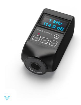
Sound pressure level: 94 dB or 114 dB Frequency: 250 Hz or 1 kHz ANSI: S1.40 IEC: 60942 class 1 The GRAS 42AG Multifunction Sound Calibrator is a portable, battery-operated precision microphone calibrator. The calibrator can be used directly on 1" microphones. Adapters for calibrating 1/2" (factory mounted), 1/4" and 1/8" microphones are included.
